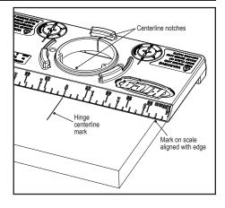
Chuck the Drill Bit into an electric drill, remove the cap from the drill bit, and install the Drill Guide/Drill Bit in the Base, turning the Drill Guide clockwise until it engages the detents. Switch on the drill, wait until it comes up to full speed, and drill the hole. Stop when the Stop Collar contacts the Drill Guide. With the drill still running, withdraw the bit and turn off the drill. Remove the Drill Guide/Drill Bit from the Base.
