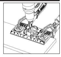
Chuck a 1% [1.5mm] drill bit into the electric drill. Insert the bit into the hinge-screw drill guides on the Base and drill pilot holes into the door. Unclamp the Base and move it to the next hinge location.
