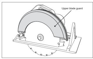
ATTENTION The Accu-Cut™ is designed for use with portable circular saws that have a metal upper blade guard. When paired with the Accu-Cut, a saw with a plastic upper blade guard may allow deflection between the blade and the base plate resulting in poor cut quality. Do not use a saw with a plastic upper blade guard with the Accu-Cut.
