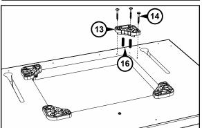
Place the table top upside down on your work bench and position an insertplate leveler **(#13)** in each corner of the opening in the table top, mating the curve on the raised portion of the leveler with the radius corner of the opening. The holes in the leveler align with pilot holes in the table-top. Fasten each leveler to the tabletop with three  $1\frac{1}{4}$ " coarse-thread screws **(#14)**.
