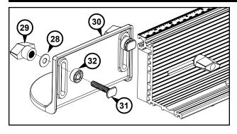
Assemble the bit guard **(#30)** using two  $\frac{1}{4}$ -20 x  $\frac{1}{4}$ " T-bolts **(#31)**, two spacers **(#32)**, two  $\frac{1}{4}$ " flat washers **(#28)**, and two T-knobs **(#29)**, as shown. Slide the T-bolt heads into the T-slot at the top front edge of the fence extrusion and tighten the knobs.
