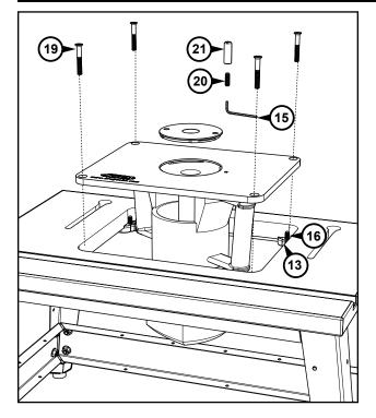
Attach the router base to the insert plate, using the screws that attached the sub-base to the router base. Depending on the thickness of your router sub-base, it may be necessary to purchase longer screws. Make certain that the screws are long enough to fully thread into the router base. If you are mounting a fixed-base router, install the motor unit in the router base.
