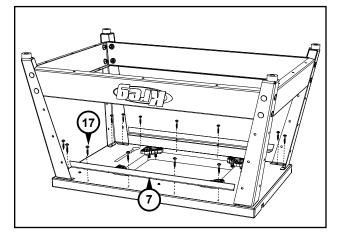
Position the legs/rails assembly on the bottom face of the router table top with the Kreg logo facing the front. (The miter-gauge track is at the front edge of the table top.) Align the holes in the top flanges of the legs with the pilot holes in the table top. Fasten the legs to the top with eight  $\frac{3}{4}$ " coarse-thread screws **(#17)**. Be careful not to strip out the pilot holes by over-tightening the screws.
