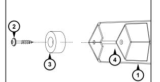
Open inner-pack box RT10180-2 and remove the legs (#1) and hardware pack. On each leg, insert a 1" coarse-thread screw (#2) through a rubber foot (#3), through the hole in the bottom of each leg, and then drive the screw into the foot support (#4) pilot hole. Be careful not to strip out the foot-support pilot holes by over-tightening the screws.
