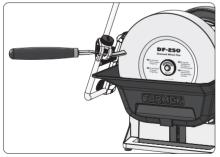
Example shows sharpening a flat bevel on a Vtool with the SVS-38 Short Tool Jig.
