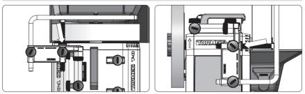
The edge angle is set by using the Micro Adjust on the Universal Support. Other settings on the MB-102 Multi Base does not affect the angle.
