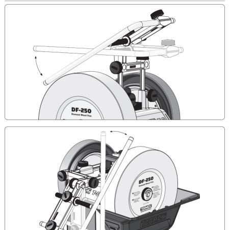
With the vertical and horizontal mounting, the sharpening position can be adjusted. This will never affect the angle setting procedure.
