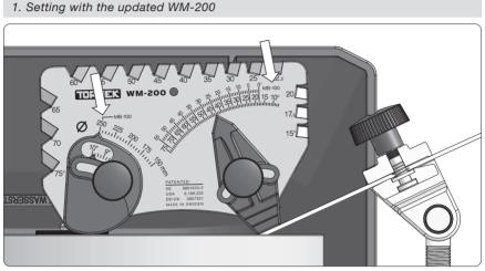
Use the top angle scale, marked with MB-100/MB-102.
