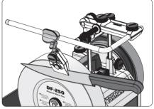
Example shows sharpening a flat bevel on a knife with the KJ-45 Centering Knife Jig.
