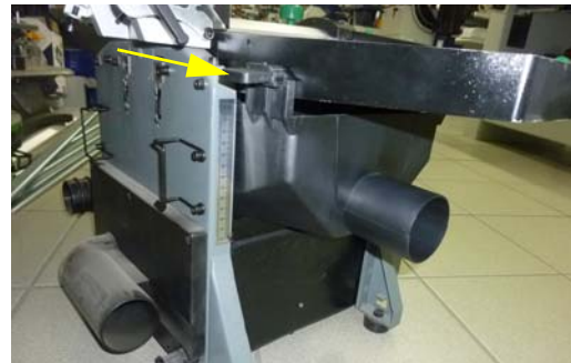
Fig. 18: Installation of the chip extraction hood
