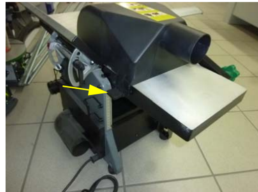
Fig. 22: Assembly of dust extraction hood
