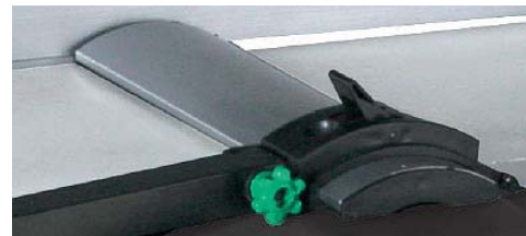
Fig. 2: Bridge protection of the planer shaft
