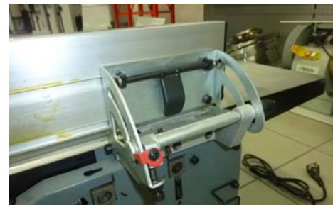
Fig. 19: Adjustment of the angle fence
