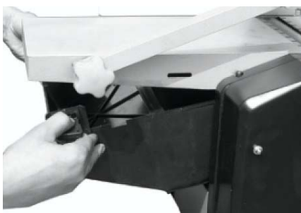
Fig. 11: Mount suction hood
