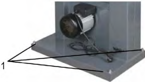
Fig. 4: Mounting on the subsurface
