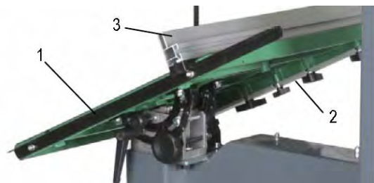
Fig. 6: Mounting the rip fence
