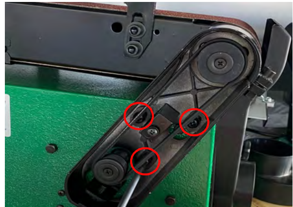
Fig. 11.2: Loosen the fixing screws of the belt holder.
