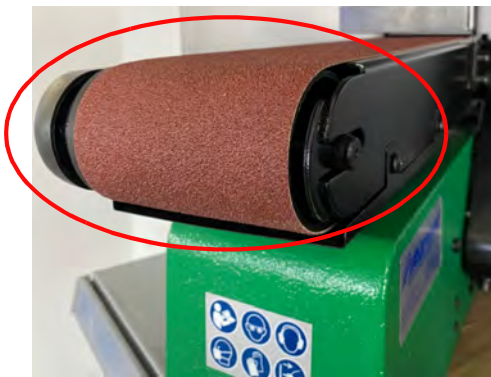
Fig. 11.1: Aligning the belt holder
