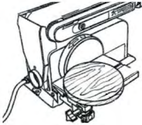
Fig. 19: Grinding round workpieces
