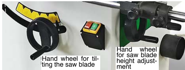
Fig. 37: Setting options of the saw blade
