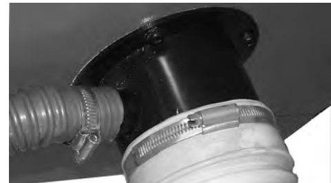
Fig. 14: Mount the suction hoses
