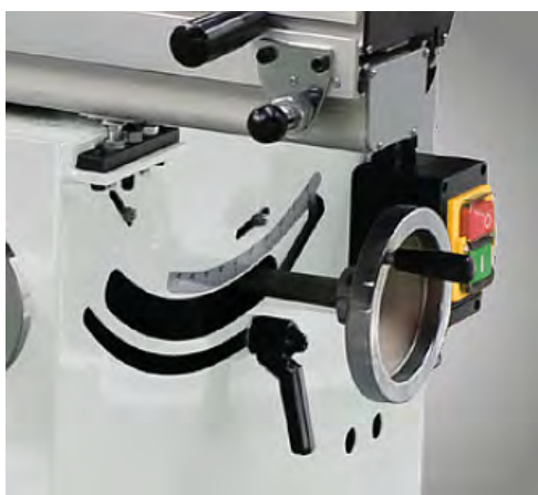
Fig. 21: Handwheel for height adjustment of the saw blade
