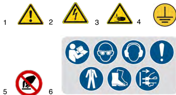
Fig. 1: 1 Warning of danger 2 Warning of dangerous electrical voltage 3 Warning of danger of crushing upper limbs 4 Grounding symbol 5 Prohibition for touching 6 Safety instructions
