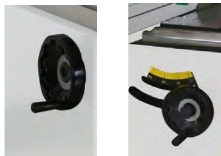
Fig. 22: Handwheel for adjusting the angle of inclination (left)
