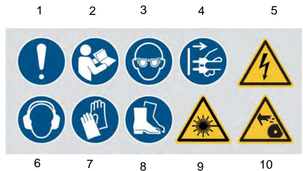
Fig. 1: Safety labels: 1 General mandatory sign | 2 Read operating instructions | 3 Use eye protection | 4 Disconnect mains plug | 5 Warning of electrical shock | 6 Use ear protection | 7 Use protective gloves | 8 Use safety boots | 9 Warning of laser beam | 10 Warning of danger due to rotating saw blade
