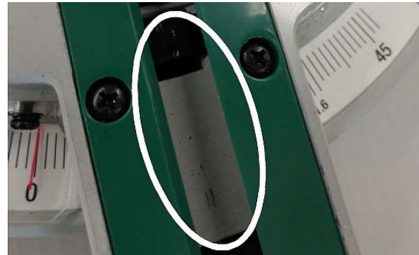
Fig. 10: Damage to the saw due to incorrect depth adjustment
