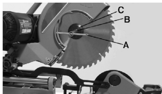
Fig. 17: Unscrew the saw blade
