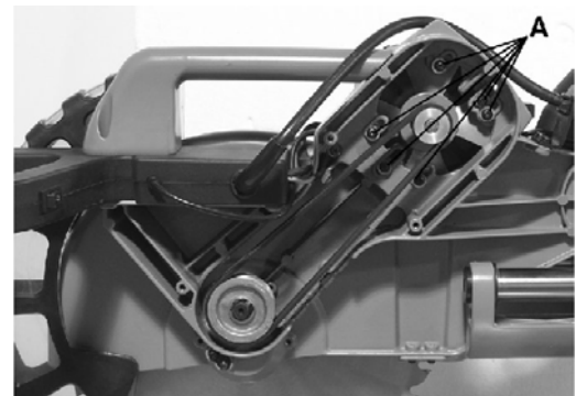
Fig. 19: Remove motor screws
