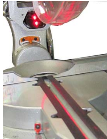
Fig. 4: Laser for marking the cutting line
