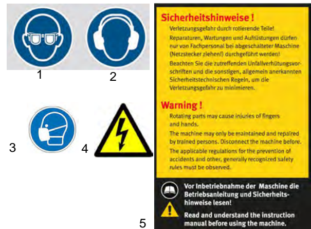
Fig. 1: Mandatory signs: 1 Use eye protection | 2 Use ear protection | 3 Wear a dust mask Safety markings: 4 Warning of dangerous electrical voltage | 5 Safety instructions
