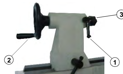
Fig. 14: Replacing the travelling tailstock centre
