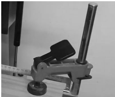
Fig. 23: Adjust the hold-down device
