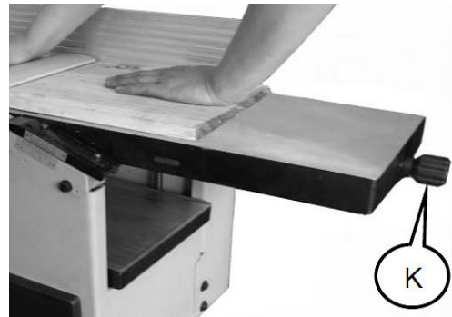
Abb. 22: Setting the chip removal
