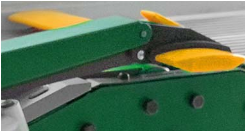
Fig. 2: Bridge protection of the planer shaft
