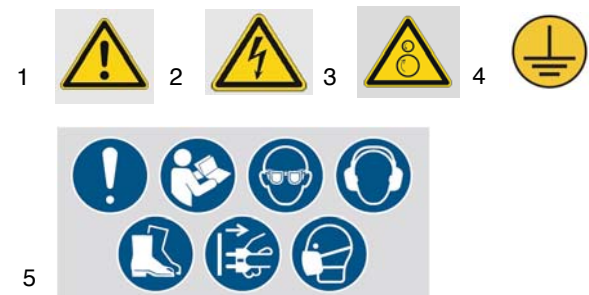
Fig. 1: Safety labels 1 Warning of danger | 2 Warning of dangerous electrical voltage | 3 Warning of danger of entanglement | 4 Ground symbol | 5 Mandatory signs
