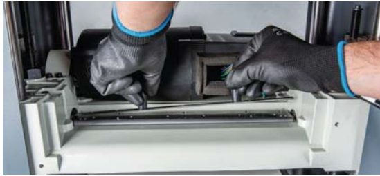
Fig. 24: Blade change with the help of magnets
