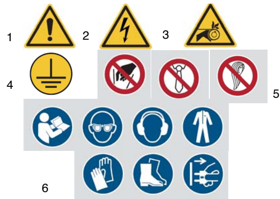
Fig. 1: Safety labels 1 Warning of danger | 2 Warning of dangerous electrical voltage | 3 Warning of danger of crushing the upper limbs | 4 Ground symbol | 5 prohibition sign | 6 Mandatory signs
