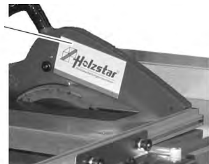
Fig. 24: Assembly of the blade guard
