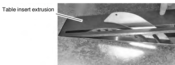
Fig. 23: Install the table insert extrusion
