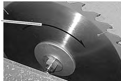
Fig. 27: Saw blade with rotary direction arrow
