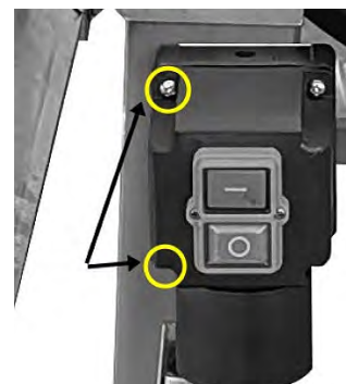
Fig. 10: Mounting On / Off - Switch
