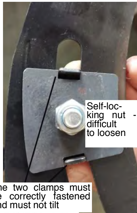
Fig. 21: Mounting riving knife part 3
