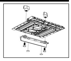
For Pulls: Insert the Drill Guides into the slots on both sides of the center hole, aligning the pointer on each Drill Guide with the dimension on the Base that matches the center-to-center dimension of your pull. The Base features center-to-center dimensions for common inch and metric pulls. Make sure the indexing peg under the pointer on the bottom face of the Drill Guide is seated in the correct indexing notch in the Base. Thread Knurled Nuts onto the Drill Guides from the bottom of the Base
