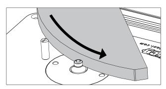
**WARNING** Use the starting pin when routing along curved edges and only with router bits that have a guide bearing. When routing along straight edges, always use the fence.
