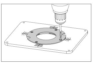
**3** Using the holes in the sub-base as guides, drill the holes in the insert plate. For best results, use a drill press. Remove the sub-base from the insert plate. Flip the plate over and countersink the mounting holes.
