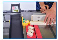
The precise 3" length of the Dado Stop allows you to accurately set the rip fence scale. Set Leg #1 gently against the blade. Reference 1.1 ALIGN BLADE (R) Set the scale cursor on the rip fence to exactly 3". Now, move your fence to desired cut width (+3"). Move the stock so that it gently touches Leg #1. Make your cut. Repeat as necessary.
