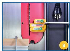
Unplug the saw. Attach the Dado Stop to your rip fence using a MATCHFIT Dovetail Clamp. Adjust the rip fence so Leg #1 is gently touching the right side of the carbide teeth at the front of the saw blade.
