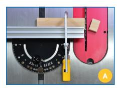
Clamp a piece of scrap to the miter gauge. Trim off the edge with the blade you will be using for your crosscut dado.
