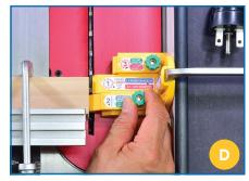
Adjust Leg #2 in front of the blade until touching the edge of the scrap trimmed earlier.
