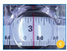
Leg #1 of the Dado Stop is exactly 3" in length. Set your rip fence scale cursor to exactly 3". Now your fence gauge will read accurately for this blade.
