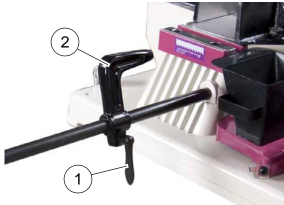
Img.4-14: Material tension, material stop
