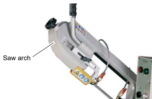
Img. 1-2: a saw blade housing with protective cover.
