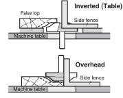
The length of the tongue on the CR/PDS1 can be increased by altering the side-fence position prior to a second pass.
