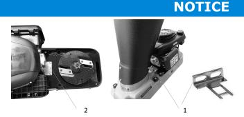
Make sure that you insert the contact plug on the hopper into the slot on the machine when placing the hopper. The machine cannot be started without this contact.
